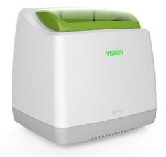
As a new generation of dynamic ESR analyzer, Vision can test up to 64 samples at the same time. With revolutionary breakthrough in technology, primary EDTA tubes can be directly used for determination and it only takes 20 minutes to obtain the results with have good correlation with the results of Westergren Method.
